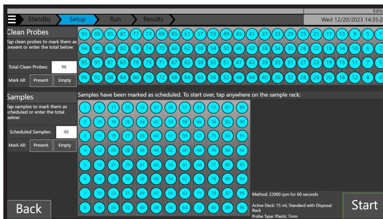
7. Perform one final check to ensure that everything matches between software and what is physically present on the Prep 96 unit. Ensure the drawer is securely fastened and the door is closed.
