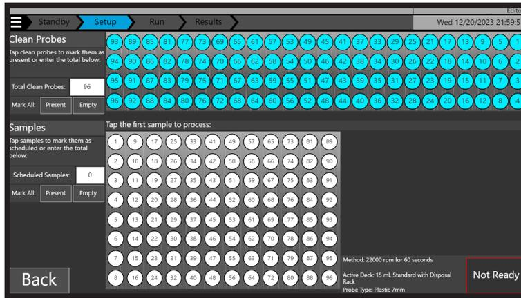
6. Select the number of samples to be homogenized using one or more of the following methods. Samples to be homogenized are indicated as light blue circles.
